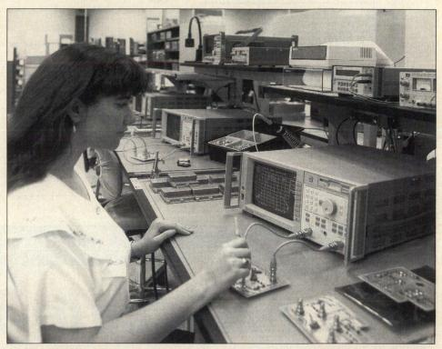
Figure 1. Fully integrated HP 8711A RF network analyzer.
