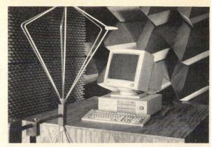
**Radiated Electric Field Testing**
